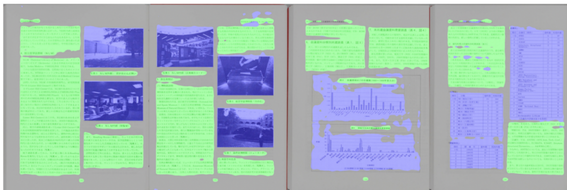
Figure 1: Results of segmentation using DeepLab V3 plus Blue areas are illustrations and green areas are text.
