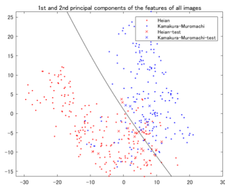
Figure 3: 1st and 2nd principal components of the features of the images of the dataset F. Dots and crosses mean training and test data, respectively. A black curve is the boundary between the features of Heian(red) and Kamakura-Muromachi(blue) periods, which was inferred by support vector machine with its box constraint 0.1.
